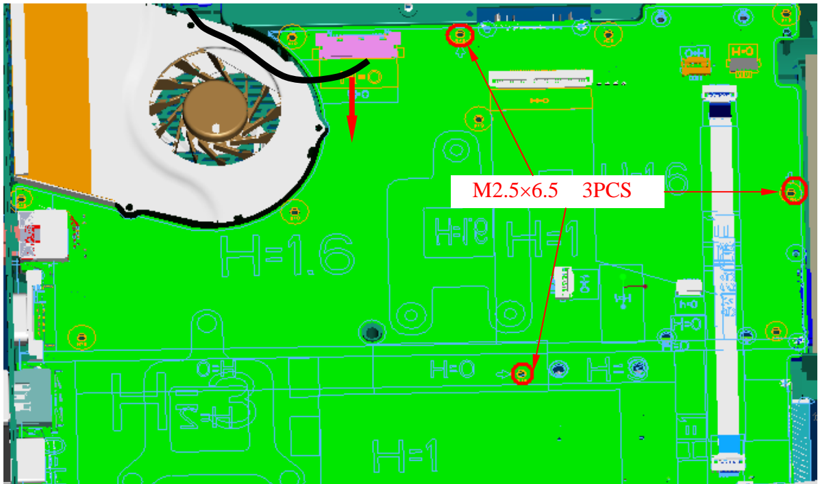
Figure 4-17-2 Remove screws for mother board
