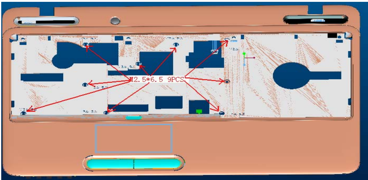
Figure 4-10-1 Remove the screws (front) and Top cover assembly
